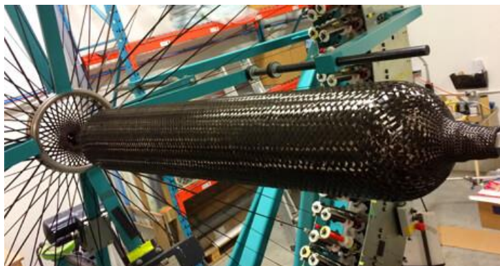
Figure 8: Tubular carbon braiding at CTT Group
