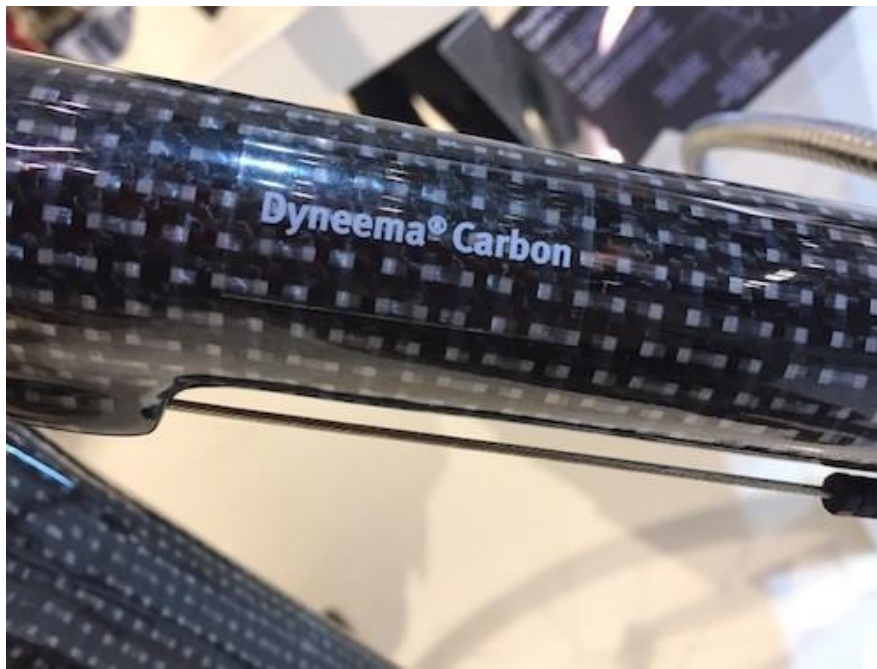
Figure 9: Bike frame made with Dyneema with Carbon fiber
